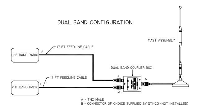
3. **Interconnect:** Refer to the dual band assembly configuration diagram. Do not tape or secure any feedlines to data or vehicle cables during installation. Remove red fit caps and connect the VHF radio to the port marked "VHF" and the UHF radio to the "UHF" port.
